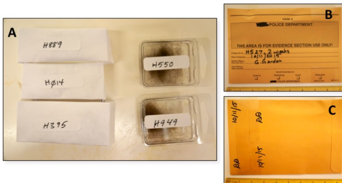
Figure 6. Photographs of packaged samples. Photo A shows a typical sample divided into aliquots for the five storage conditions. Photos B and C show the sealed evidence envelope.
