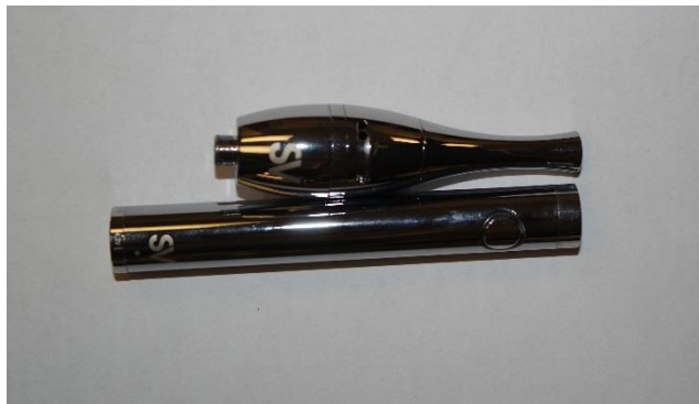
Figure 1. Source Orb 4 E-cigarette and Atomizers
