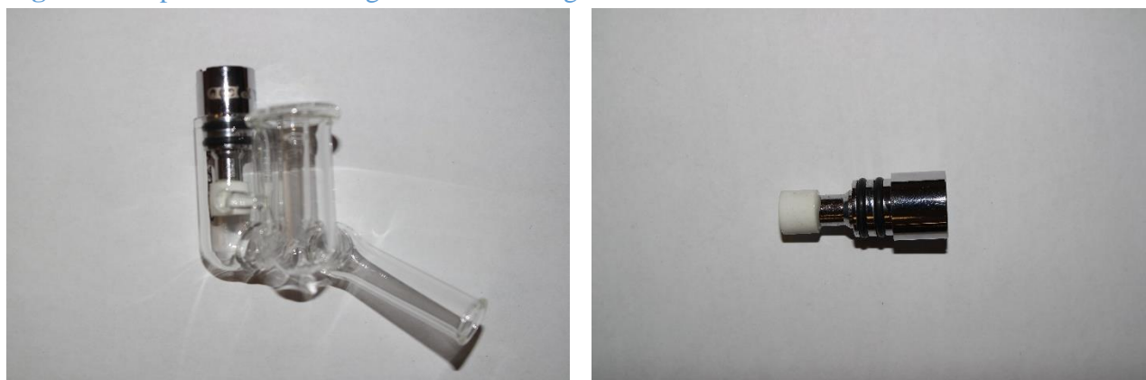
Figure 4: Vaped Vubbler E-Cigarette with a single titanium coil with Ceramic Atomizer
