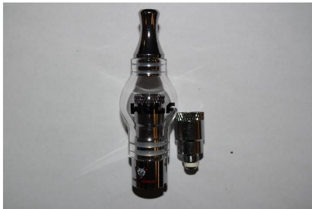
Figure 3. Wulf Mod E-Cigarette and the Dual Coil Ceramic Atomizer
