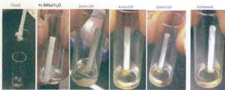
Figure 9: Photodissolution of PHEMA-50%-NBS+PEG=1:1 swab material.
