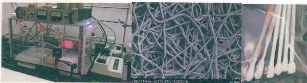
Figure 7: GE-GRC's electro-spinning device and microscopic image of swab fibers.
