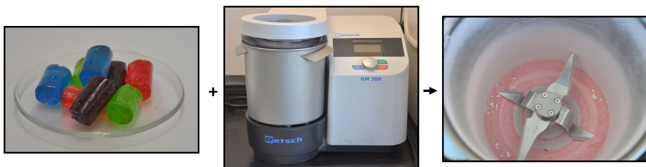
Figure 2. Cold homogenization of hard candy using industrial grade food homogenizer and dry ice
