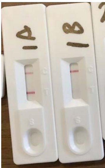
Figure 10. Competitive lateral flow immunoassay cassette developed by CDC-NIOSH for detection of methamphetamine at a concentration of 50 ng/100 cm 2 . Sample 1A was taken pre-cook and sample 1B was taken from the same location post-cook. Two red lines indicate the absence of methamphetamine in the sample. One red line indicates the presence of methamphetamine in the sample.
