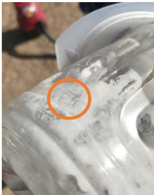
Figure 23. A hole formed in the One Pot reaction vessel of the second camp fuel cook due to repeated expansion and relaxation of the plastic.
