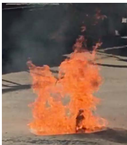
Figure 80. The first One Pot burn during the fire control study. As can be seen, the bottle broke open during the fire, causing a puddle of ether to surround the burning bottle and ignite.
