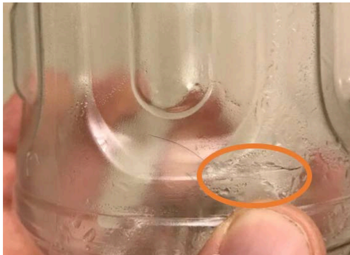
Figure 24. A hole formed in the One Pot reaction vessel of the final camp fuel cook due to repeated expansion and relaxation of the plastic.
