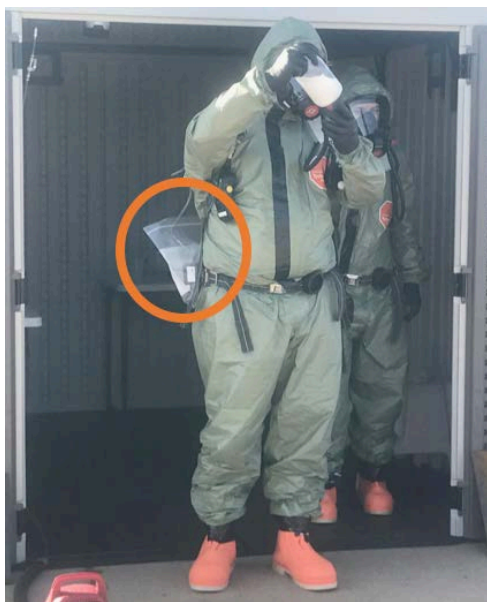
Figure 11. An active air sampler fitted to a researcher as they performed a One Pot methamphetamine cook.
