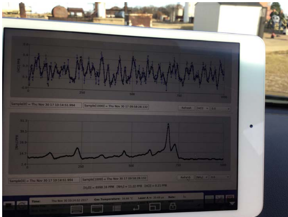
Figure 54. Bottom plot depicts ammonia peaks captured during 6 vehicle passes during the Thursday morning camp fuel cook. A new rising ammonia edge begins at far left during vehicle tangential approach to rear of cook shed (seen in top right) during this 7 th driving pass as viewed on the 15-minute data screen.
