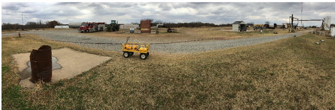
Figure 57. Yellow cart containing battery-powered ICOS NH 3 -HCl gas analyzer and external vacuum pump placed 40 meters downwind from cook shed during Tuesday afternoon camp fuel cook.
