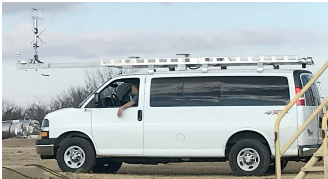
Figure 16. The GMAP unit operated by EPA-NEIC. On-board instrumentation includes an ICOS, PID, DUVAS, GPS, a weather station, and an air canister collection mechanism.
