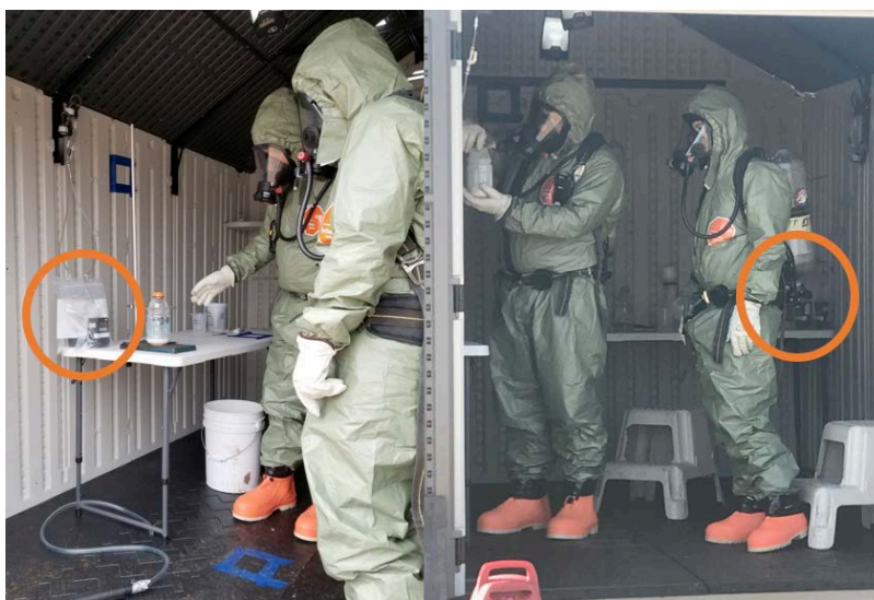
Figure 12. Locations of 4 out of 5 active air samplers. Two samplers were placed in each location designated by the orange circles. Two samplers were located left of the active One Pot methamphetamine lab and two samplers were located behind and to the right of the researchers performing the One Pot methamphetamine cooks.
