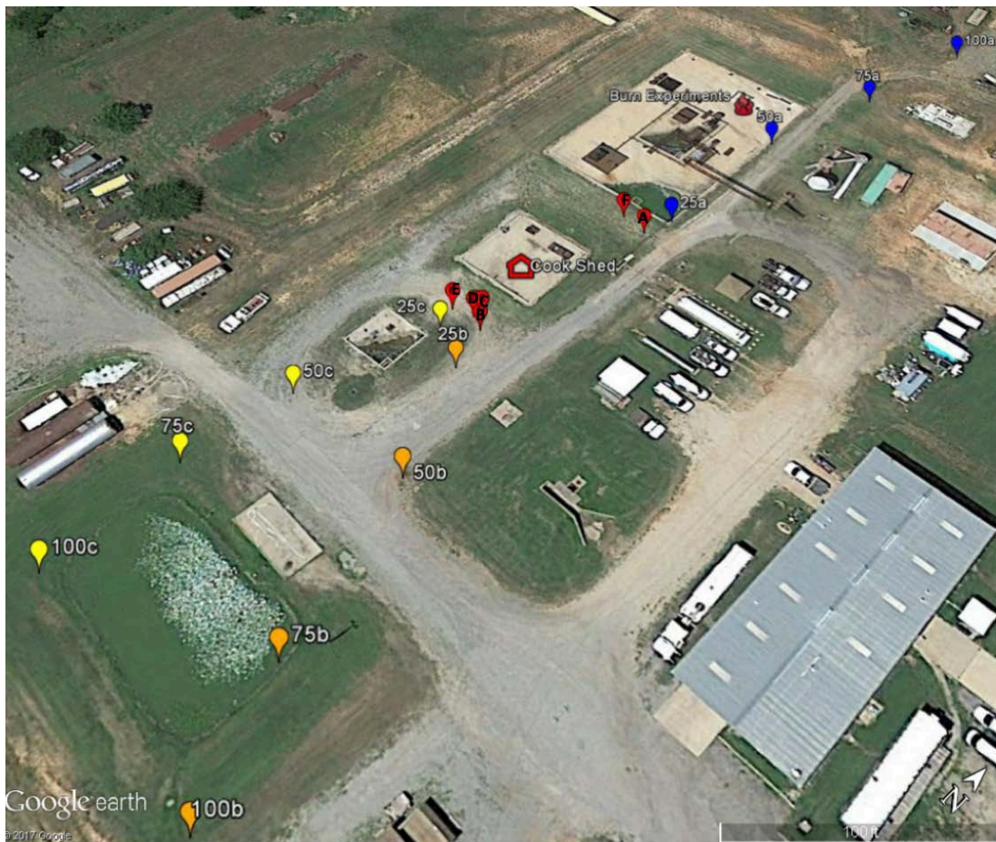
Figure 17. GMAP unit and SPod sampling locations at the Oklahoma State University Fire Research and Training Center.
