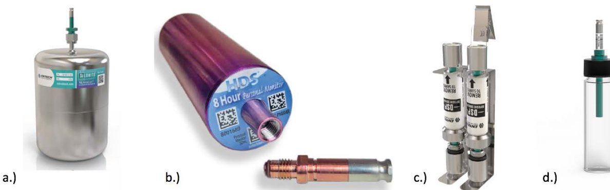
Figure 13. Passive air monitors provided by Entech Instruments for the shed interior air monitoring study. a.) 1L Minican™ vacuum canister, b.) Helium diffusion sampler (HDS) personal monitor, c.) A set of diffusive sorbent pens (DSPs), one packed with Carbo Pack X and one packed with Tenax, and d.) a 40 mL screw-top grab sampler.
