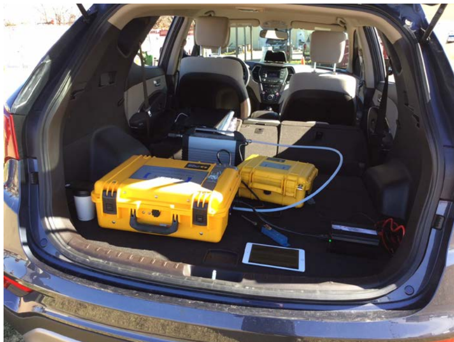
Figure 20. Configuration of battery-powered ICOS NH 3 -HCl gas analyzer (foreground), vacuum pump (gray), battery pack (yellow-right) as positioned in moving vehicle during data-logging. Trace ammonia detected from vehicle exhaust was dampened or eliminated by opening all vehicle windows when vehicle was in motion or by shutting off the engine when parked as shown.
