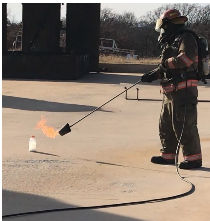
Figure 22. All One Pots were ignited by a trained firefighter wearing turnout gear and SCBA. One Pots were ignited with a propane torch as shown.
