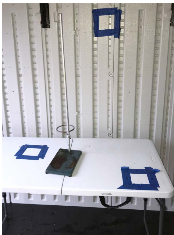
Figure 8. Three of eleven 10 x 10 cm (100 cm 2 ) sampling locations selected within the One Pot methamphetamine cook shed.
