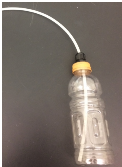
Figure 5. A typical hydrogen chloride gas generator, comprised of a plastic bottle with a hole in the cap and a hose protruding from the hole.
