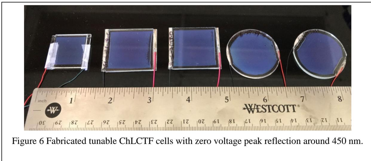
Figure 6 Fabricated tunable ChLCTF cells with zero voltage peak reflection around 450 nm.
