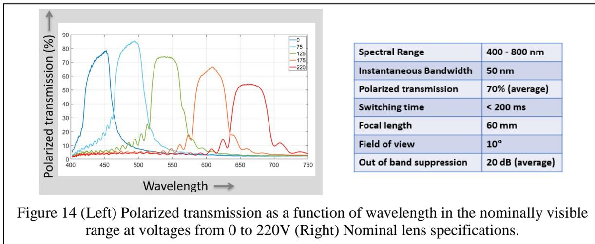
Figure 14 (Left) Polarized transmission as a function of wavelength in the nominally visible range at voltages from 0 to 220V (Right) Nominal lens specifications.
