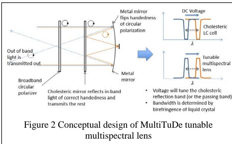
Figure 2 Conceptual design of MultiTuDe tunable multispectral lens
