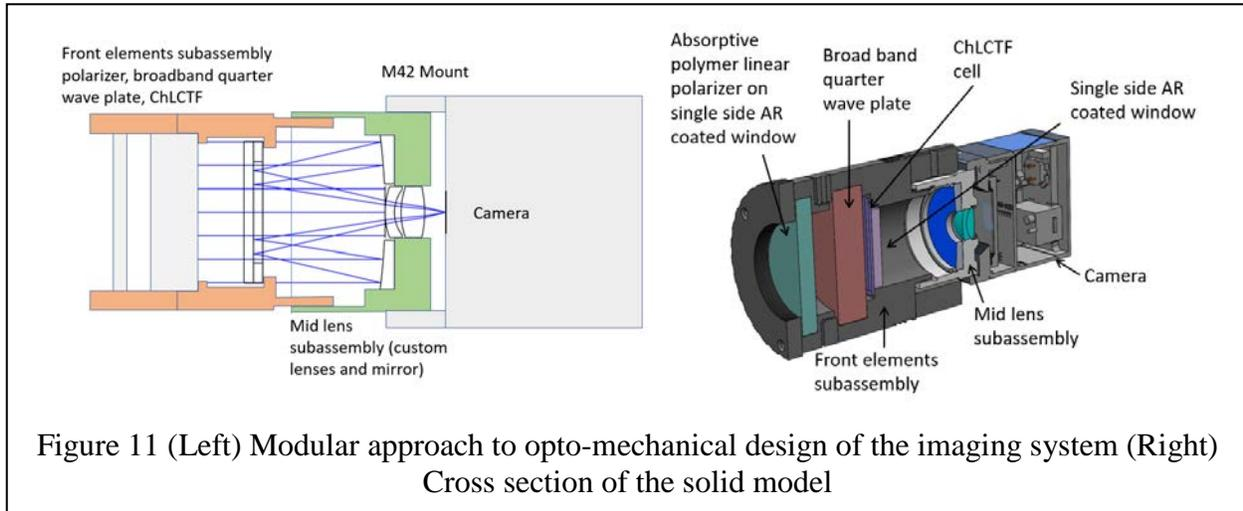
The mid sub-assembly consisted of the custom aspheric reflector with a metal coating, and two custom spherical lenses, assembled with high precision mechanical tolerances.
