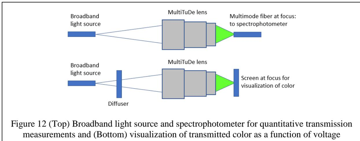
Figure 12. We also used a screen with broadband light source for visualization of color transmitted by the lens as a function of applied voltage.
