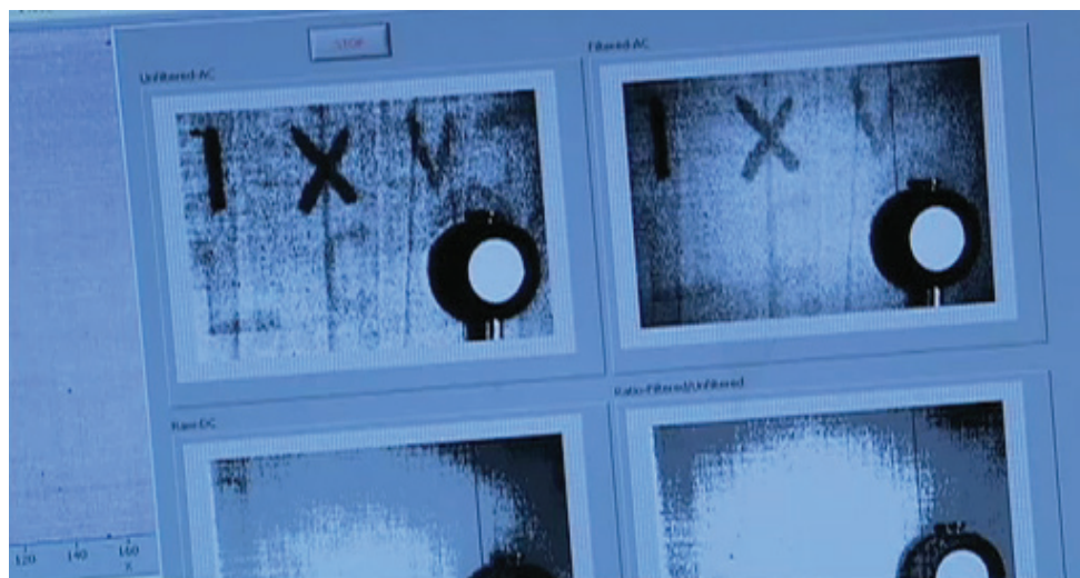
Example images of blood stains captured using the prototype IR camera that was developed with the support of NIJ funding.
