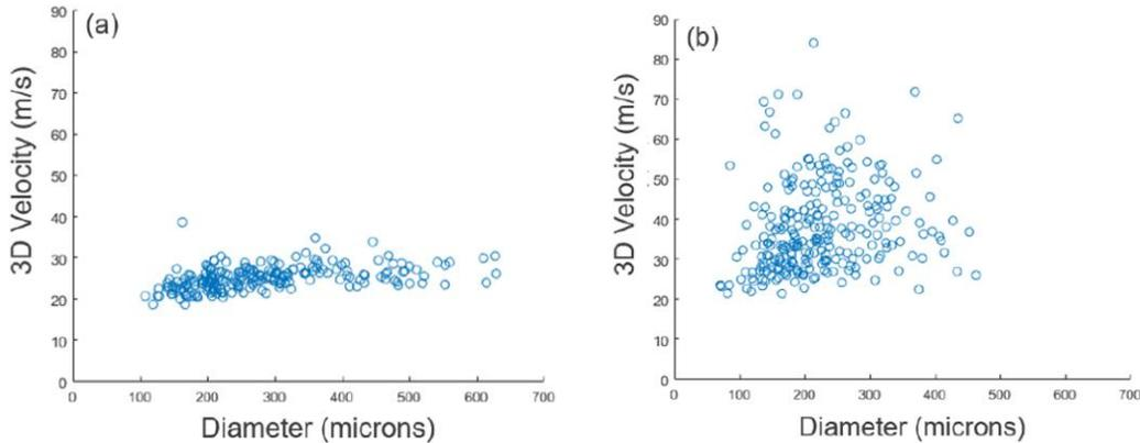
Figure 3: Droplet size-velocity scatter plots showing the distribution resulting from blunt impact on a (a) thin film of water and (b) a thin film of blood. Reproduced from (Das Diss. 2019).
