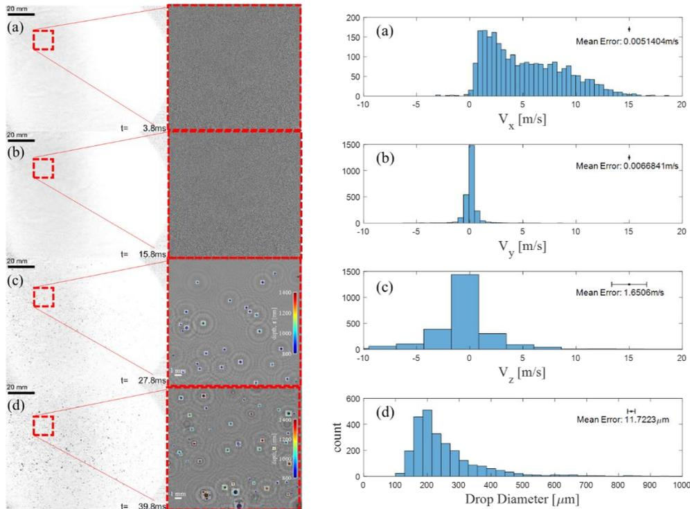
Figure 4: (Left) Location for monitoring backspatter from a .22-caliber rifle bullet approximately 0.6 m from the target. Insets show refocused holograms with identified droplets. Using particle-linking approaches in Sandia's HoloSand v1.0 code, individual droplet parameters are determined. A total of 2500 particles are identified, with 3D velocities and diameters shown in the histograms of the right panel (Sliefert Diss. 2020, Michael et al. in preparation).
