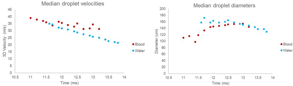
Figure 2: Median droplet velocities and diameters resulting from a blunt impact on a thin liquid film of blood and water. Reproduced from (Das Diss.2019).
