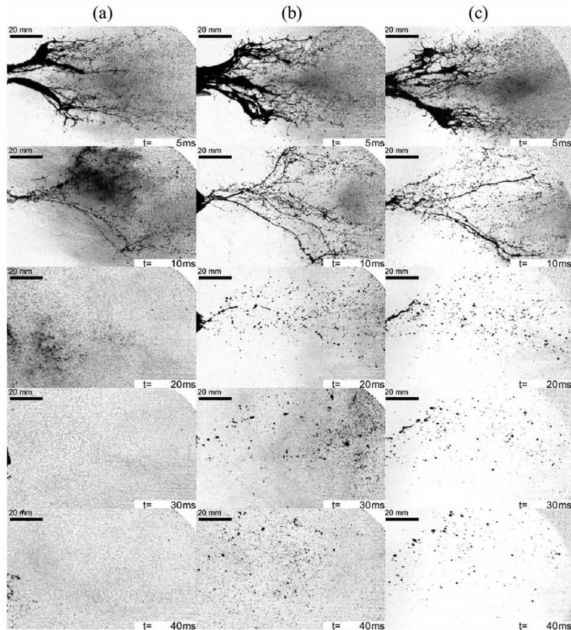
Figure 1: Muzzle gas interaction cases over increasing muzzle gas distances. Distance from muzzle to blood source is (a) 65 cm, (b) 125 cm, and (c) 300 cm. Reproduced from Sliefert et al. (2021).
