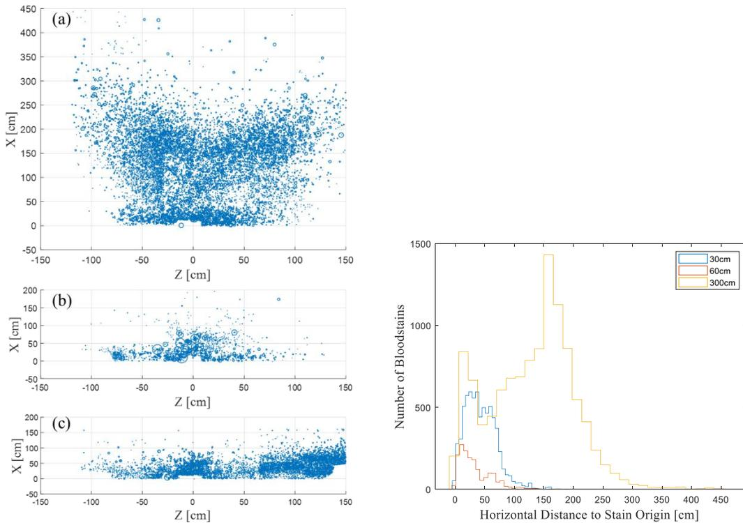
Figure 5: (Left) Bloodstain pattern collected on butcher paper on the floor in a backspatter configuration. Three cases are shown for muzzle gas standoff distances of 30, 60, and 300 cm corresponding the shadowgraphy images shown in Figure 1. (Right) The number of bloodstains presented as a histogram with the horizontal distance from the stain to the origin. (Sliefert Diss. 2020, Michael et al. in preparation).
