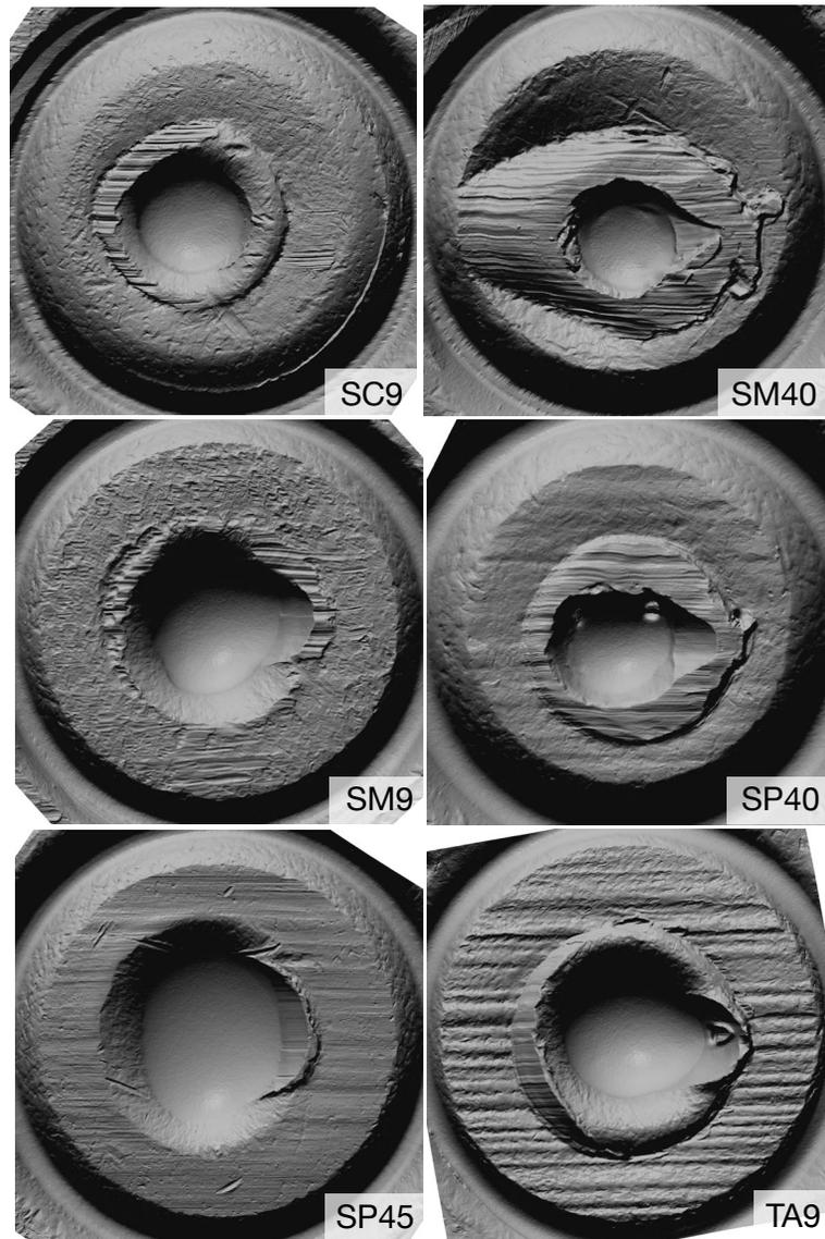
Figure 10: **Test Set Cartridge Cases (Part 2)**. Scans of one test fire from the second six firearms in the test set (Table 1) labeled by the firearm's short name.
