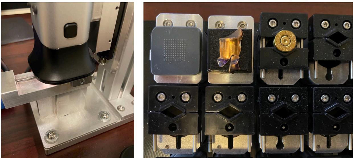
Figure 12: **Scanning Damaged Bullets.** (Left) The bullet holder positioned in the portable scanner under the scanning head (black). Damaged bullets can be mounted on a plastic base (not shown) and placed under the scanning head in place of the bullet holder shown. (Right) In the desktop scanner a bullet fragment can be positioned mounted on a flat holder in the desktop scanner's scan tray.
