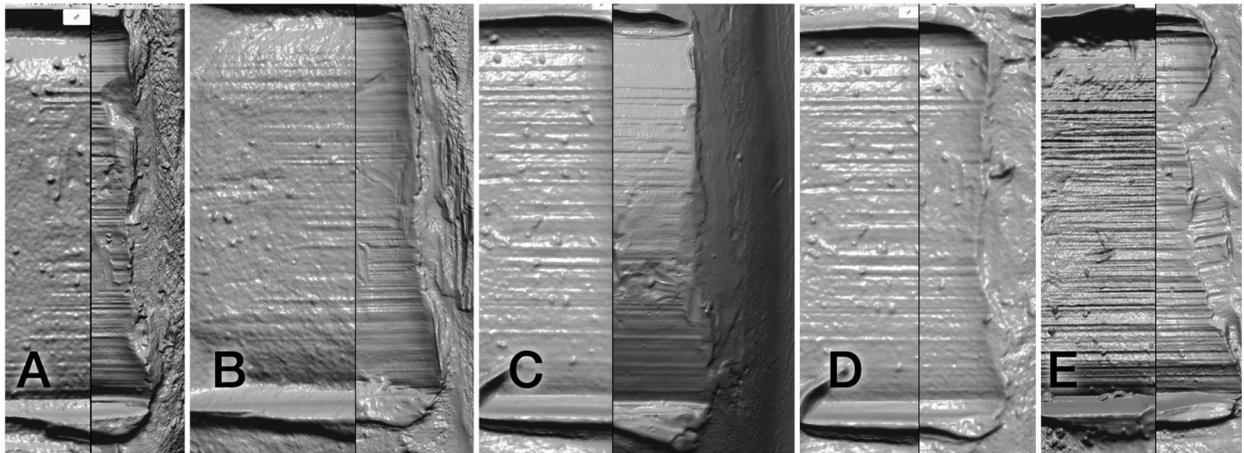
Figure 13: **Damaged Bullet Scanning.** All comparisons shown are KMs (non-exact) from the Beretta (BE40) firearm. (A) Left: Portable Pristine. Right: Desktop Pristine. (B) Left: Portable Mushroomed. Right: Desktop Pristine. (C) Left: Portable Fragment. Right: Desktop Pristine. (D) Left: Portable Fragment. Right: Portable Pristine. (E) Left: Desktop Fragment. Right: Desktop Pristine. Most LEAs are shown flattened.
