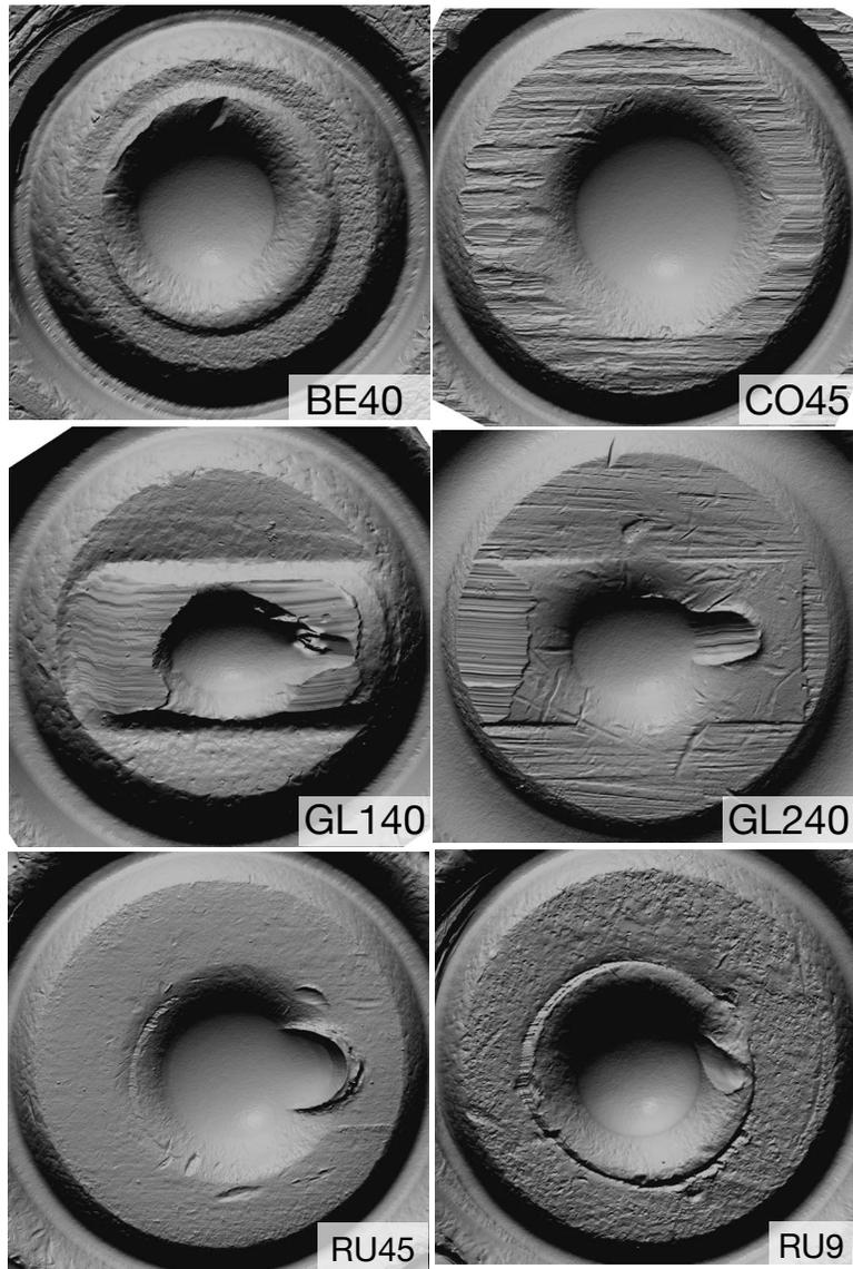
Figure 9: **Test Set Cartridge Cases (Part 1)**. Scans of one test fire from the first six firearms in the test set (Table 1) labeled by the firearm's short name.
