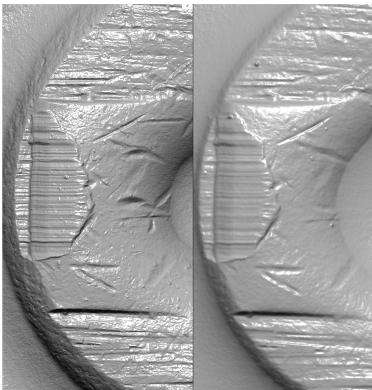
Figure 6: **Desktop and Portable Scan Quality.** Scans of the same Glock test fire are shown as collected on the desktop scanner (left) and the portable scanner (right).
