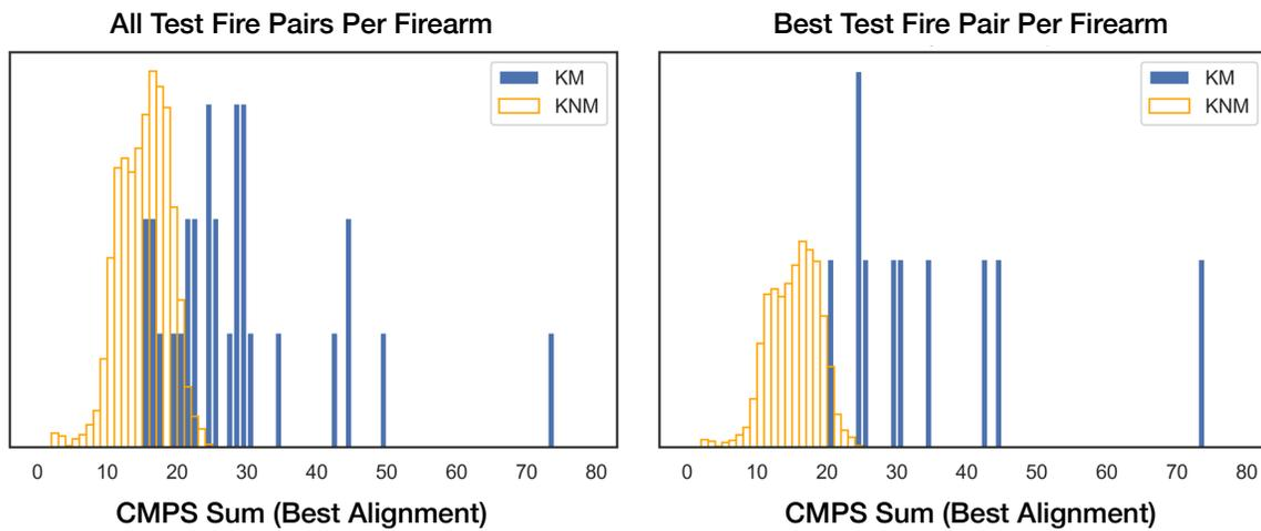
Figure 11: **Bullet Score Distributions.** (Left) CMPS Sum scores at the best alignment for all test fire pairs. (Right) CMPS Sum scores at the best alignment for the highest scoring test fire pair for each pair of firearms.
