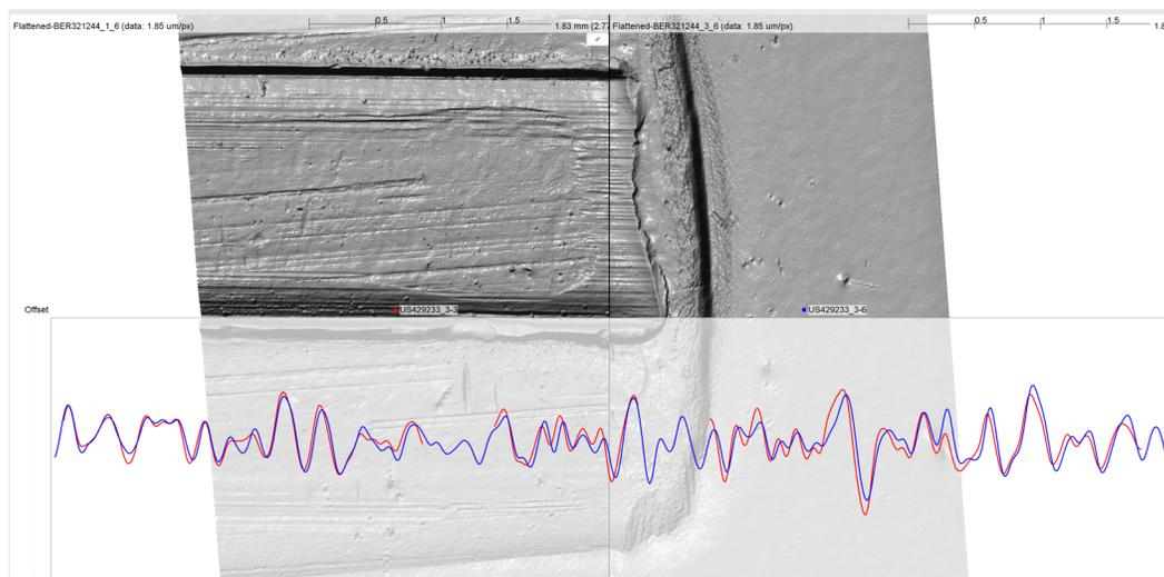
Figure 8: **Matched LEA.** (Top) Flattened view of matched LEAs from two Beretta test fires. (Bottom) Extracted and aligned striation profiles from each LEA. The blue profile is from the right LEA and the red profile is from the left LEA. The blue profile appears as a solid line. The red profile appears solid where it matches the blue profile and dashed where the CMPS algorithm did not identify significant agreement.
