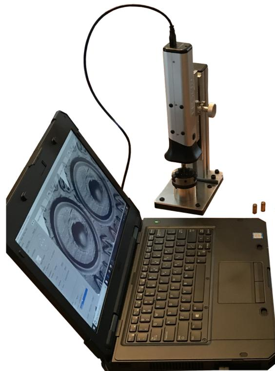
Figure 5: **Portable Scanner.** The portable scanner is approximately 12” tall and uses a laptop for scan acquisition and power. A small cartridge case holder consistently positions each cartridge case under the gel pad and imaging optics. When used for bullet scanning the bullet holder (Fig. 2) can be placed under the gel pad an imaging optics.
