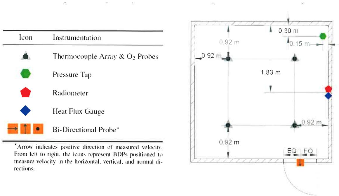
Figure 1. Schematic of the compartment floor plan with location of fixed instrumentation arrays identified.
