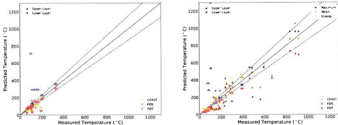
Figure 2. Comparison of Layer Temperature Predictions to Experimental Data Collected in Compartment Experiments with Steady State Gas Burner Fires (left) and Furniture Fires (right).
