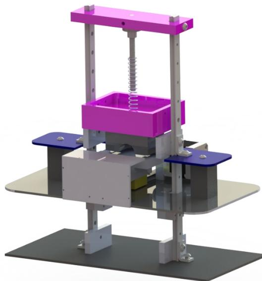
**Figure 1** Sketch of fingerprint press.
