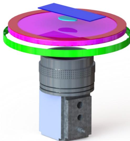
**Figure 2** Exploded view of the large-area TIR illumination system illuminating the fingerprint on a microscope slide (*dark blue*) imaged from below by a CCD camera.
