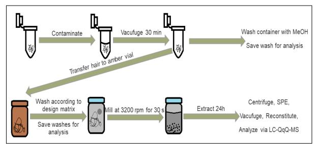
Figure 1. Schematic of decontamination DoE procedure.
