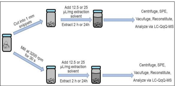
Figure 2. Schematic of pretreatment DoE procedure.
