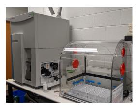
Figure 1: ICP-MS and autosampler used for analysis of digested Al samples.
