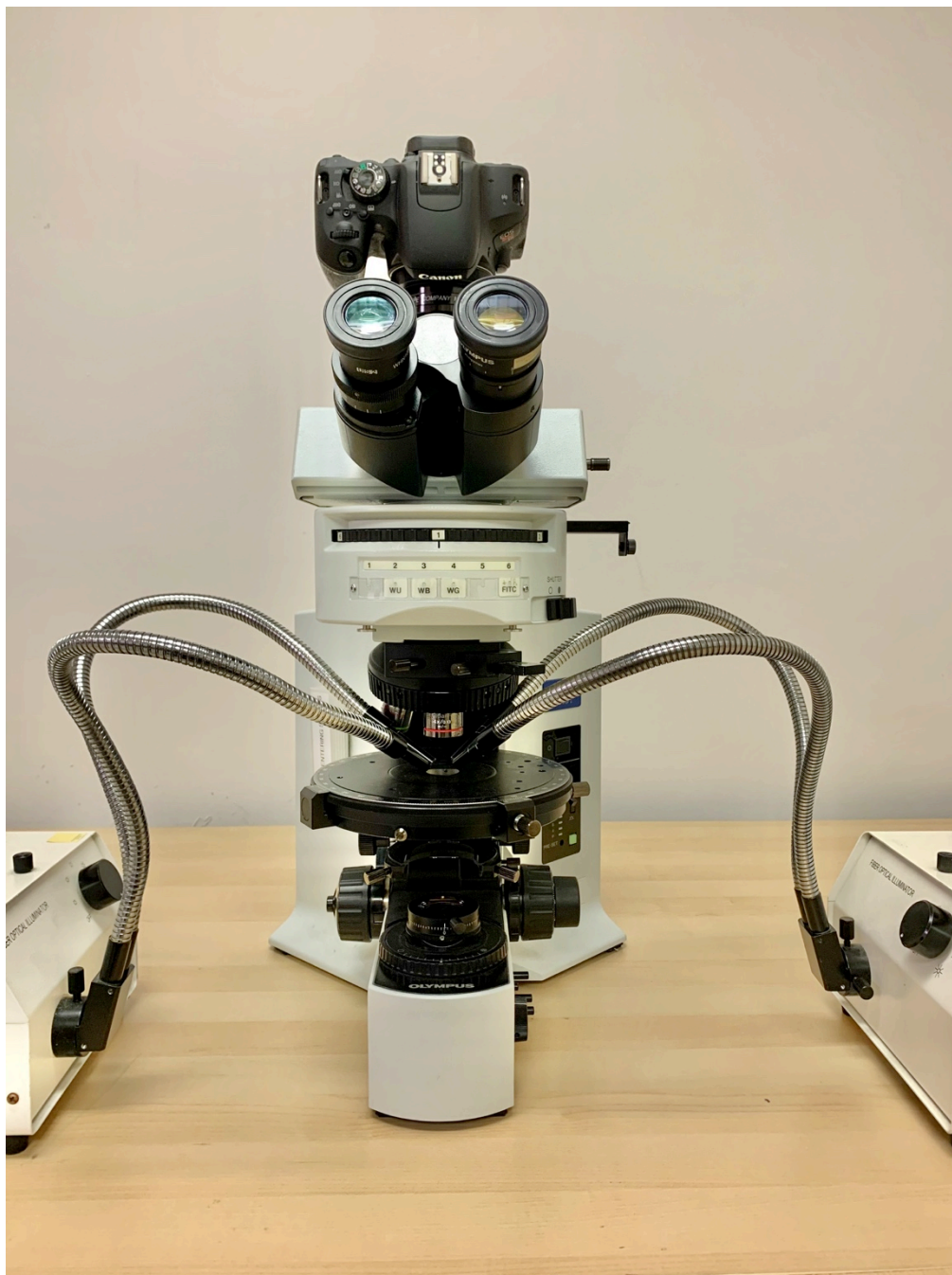
Figure 3. Microscope, illumination, and camera arrangement used to take images for the photomicrographic photomontages obtained in this research. This convenient setup utilizes a conventional PLM and the use of various illumination conditions. All photomicrographs were taken with a digital, single-lens reflex camera paired with commercially available image-capture software.
