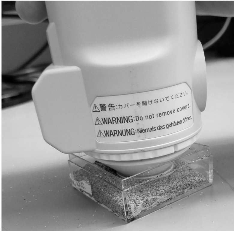
Figure 30: Placing instrument in evidence container for color measurement
