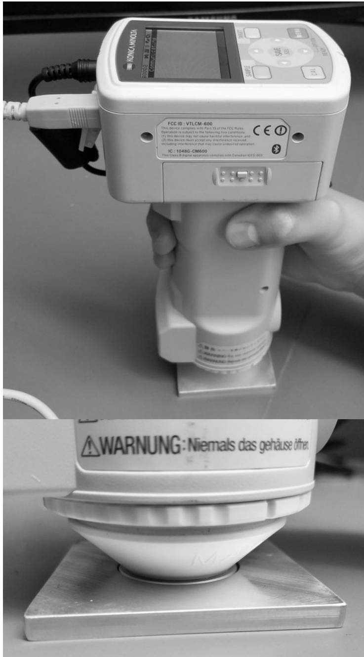
Figure 28: Placing instrument in sample holder for color measurement
