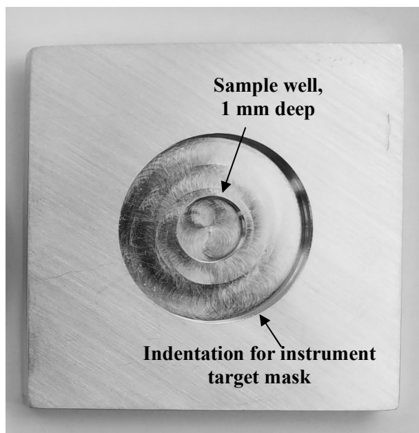
Figure 27: Custom aluminum sample holder, 1mm deep
