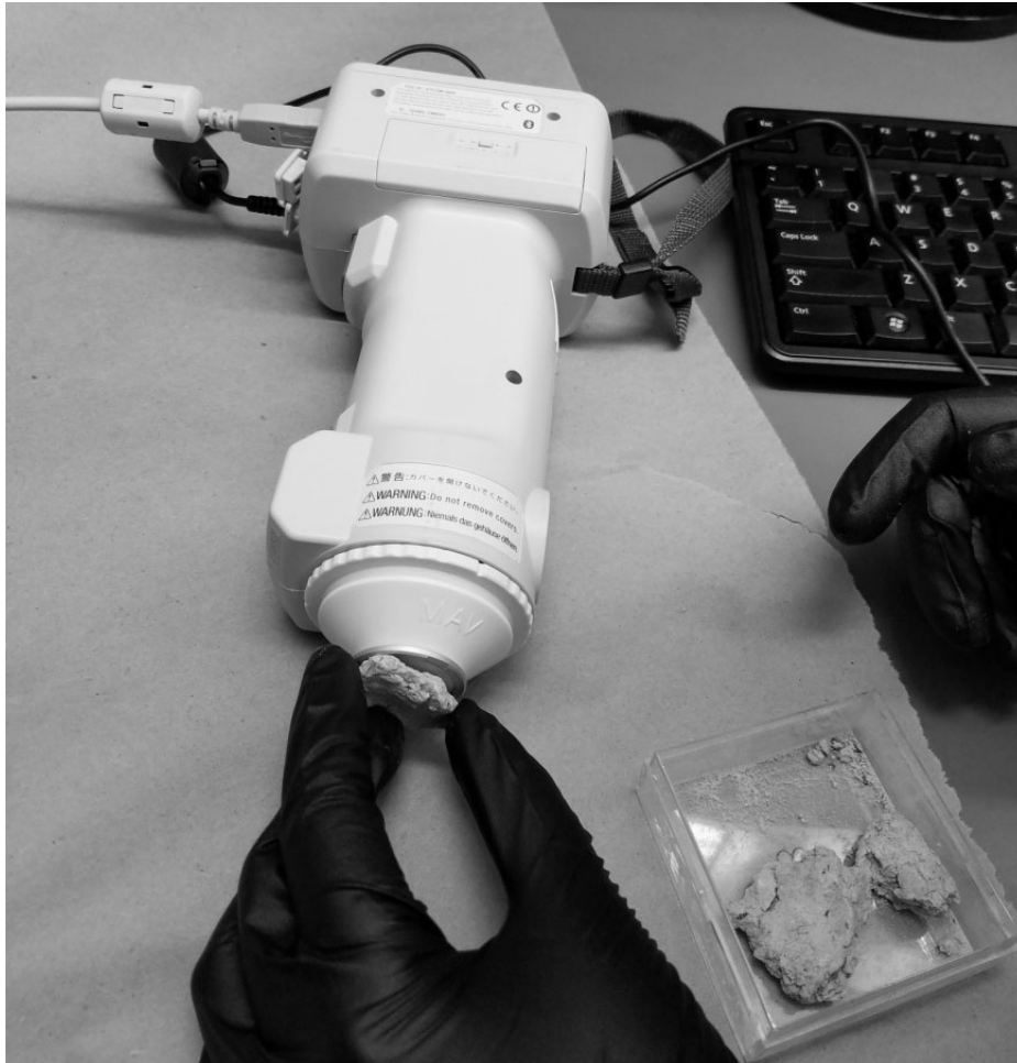
Figure 29: Placing aggregate for color measurement
