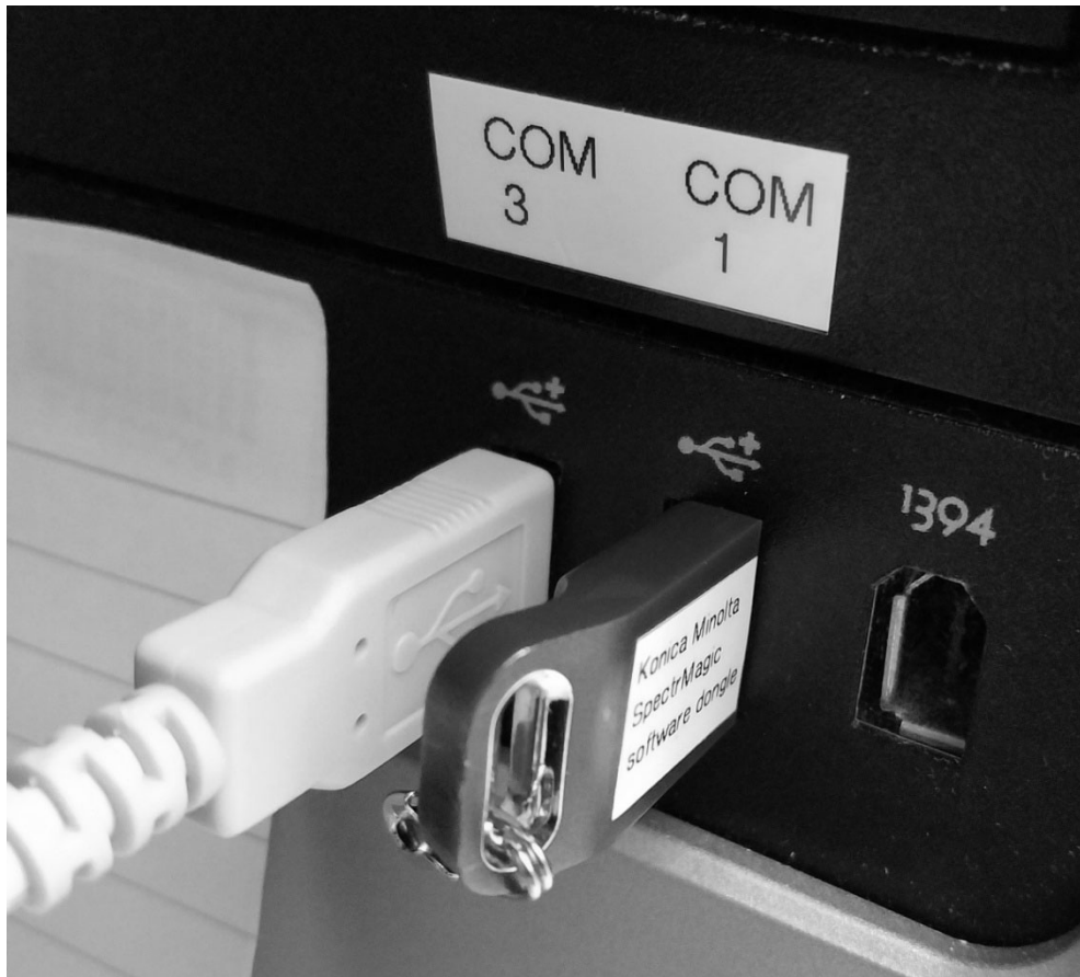
Figure 14: USB ports on front of Soil Lab computer labeled by COM port
