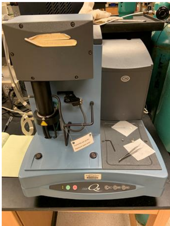
Figure 8: TA Instruments TGA Q50 device utilized to perform Thermogravimetric Analysis.
