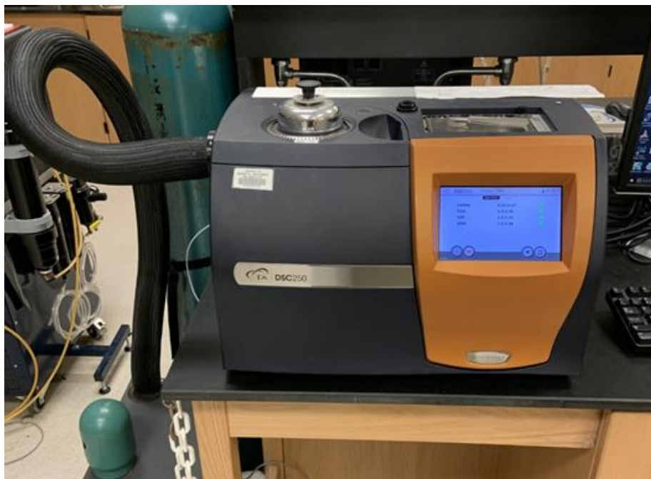
Figure 9: TA Instruments DSC250 device utilized to perform Differential Scanning Calorimetry.
