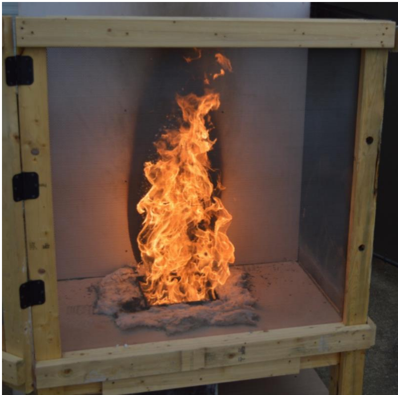
Figure 6: Test apparatus constructed for the diffusion burner tests
