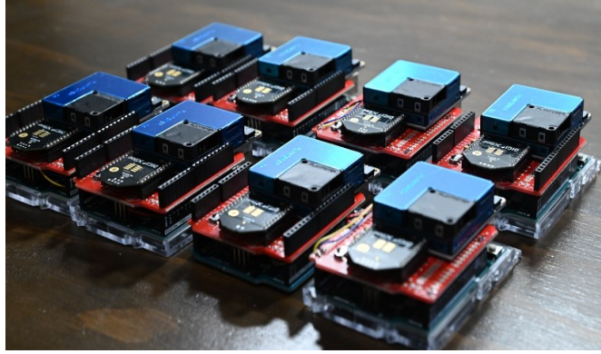
Figure 4. Custom-made particle counting devices. Photograph courtesy of Matthew Staymates
