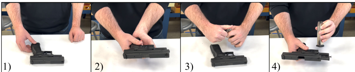
Figure 10. Photographs of mock crime scene handling of the firearm procedure: 1) firearm in hand, 2) release magazine and rack slide and repeat, 3) load ammunition, and 4) insert magazine.
