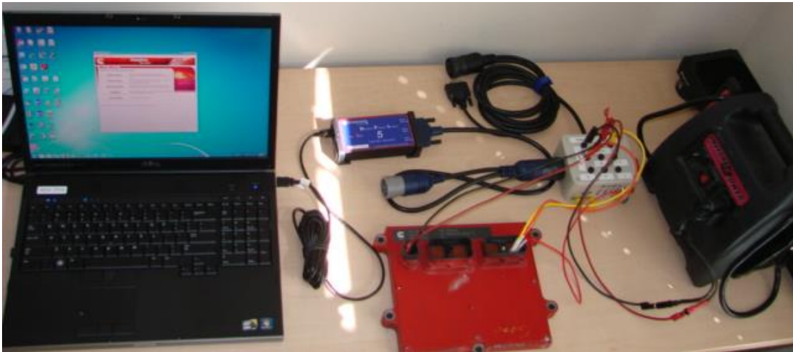
Figure 2: Bench download from a Cummins ECM.
