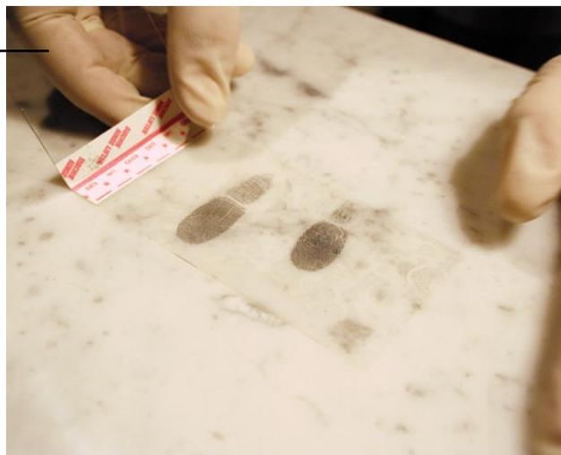
**FIGURE 8-18***Hinge lifter.*
