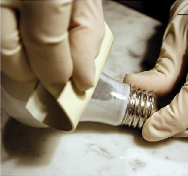
**FIGURE 8–19***Rubber-gelatin lifter.*
